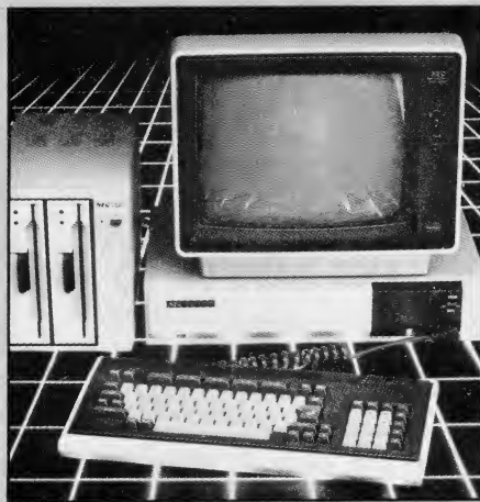
NEC PC-8800 bundled system includes system unit, keyboard, dual disk drives, and monochrome monitor.
